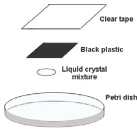
Gently warm or cool the liquid crystal mixture from the tape side while viewing the top of the Petri dish. Note the temperature when changes occur. What happens?
