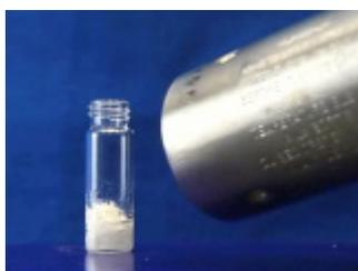
Melt the solid in a sample vial using a heat gun.
