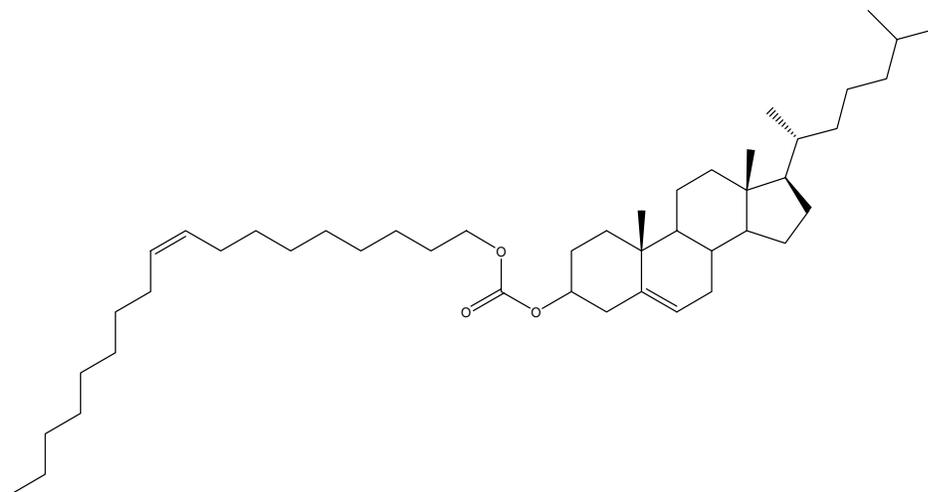
These cholesteric-nematic liquid crystals reversibly change color as the temperature changes. One of the principal advantages of liquid crystals is their ability to map out thermal regions of different temperature. Liquid crystal films exposed to the atmosphere will decompose slowly; their lifetime can be extended by encapsulation.
