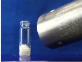
Heat the sample with the heat gun to melt the liquid crystal mixture.
