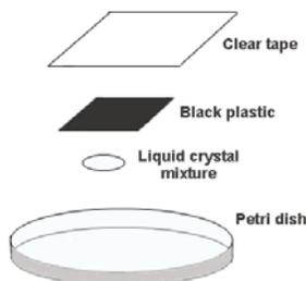
Use a wood applicator stick to place a small amount of the liquid crystal mixture to the inside of a Petri dish. Place a piece of black plastic, approximately 2.5 cm square, on top of it and seal it in place with a 5 cm square of clear plastic shipping tape.
