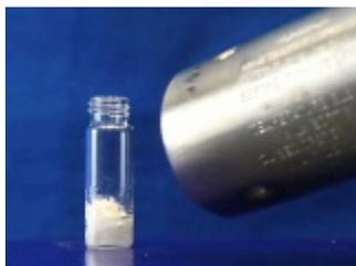
Melt the solid in the vial using a heat gun.
